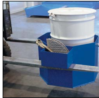
Transport Sump with Forklift Attachment
