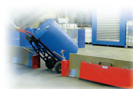
When open, store the barrier close to the mounting piers for quick, easy deployment in the event of a spill.
