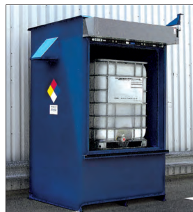
Lockers for 1-2 IBC, 2-hour fire rated design is constructed with UL Approved firewalls. Roll-up doors includes fuse link and will automatically close in case of fire.
