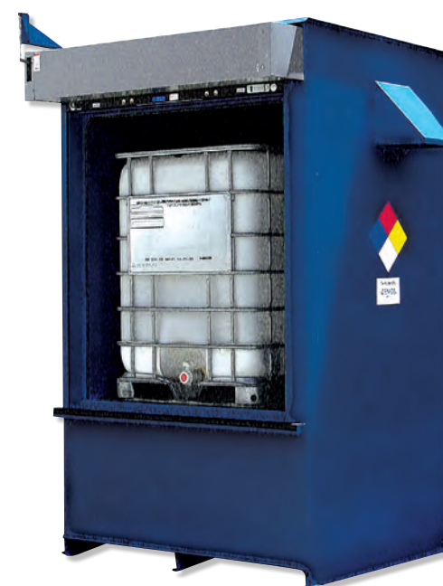
2-hour Fire Rated IBC Locker with roll-up door. Door includes fuse link and will automatically close in case of fire.
