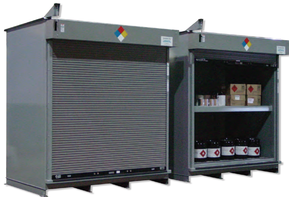
Optional fixed shelf provides for storage of small packages of flammables. Automatic fire doors remain open for access to packages and will close in case of fire in or outside of the Locker.
